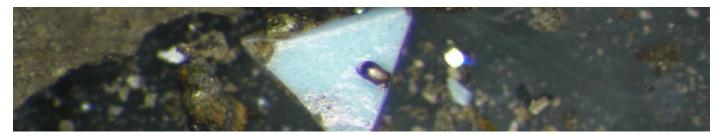
Optical image of an unknown particle observed within a sample of debris. The particle was established to be a traceable ceramic meaning the origin was quickly established.
